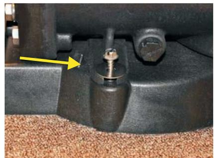
5. Tighten the screws until it just touches the base and then turn it an additional 1/4 turn. Do not over tighten the screws in the plastic base. If you see the stainless washer bend then that is too much.
