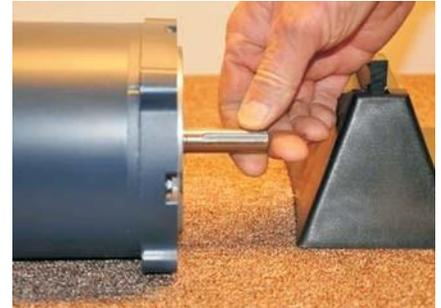
8. Install the motor by guiding the motor shaft inside the pump coupling. Make sure the key way aligns with the set screws.
