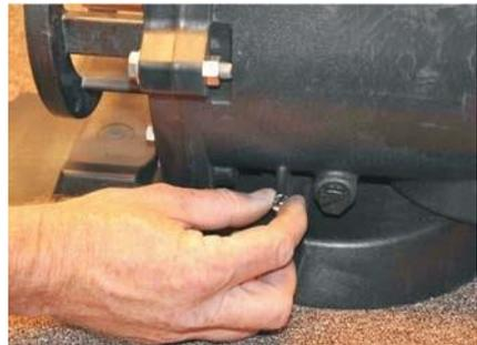
4. Make sure the pump is straight in the base and the screws are aligned vertical before tightening.
