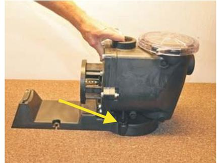
3. Place the stainless steel flat washers over the base flanges on each side of the pump. Insert the two stainless steel screws and start the two base mounting screws by hand.
