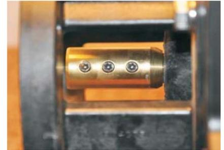
7. Rotate the motor shaft until the key way is at the same 45 degree angle to align with the pump coupling set screws. Apply a small amount of never seize or grease to the motor shaft before inserting into coupling.
