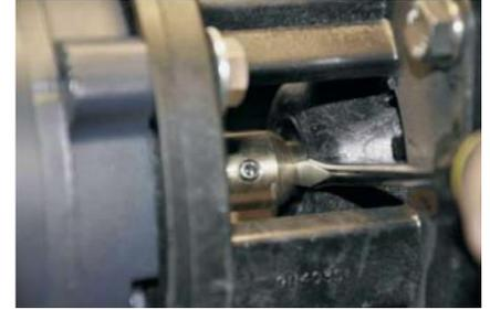
12. While holding the pump shaft in position with the screw driver, insert a 1/8" Allen wrench into one of the set screws and tighten. You can then remove the screw driver and tighten the other two set screws.
