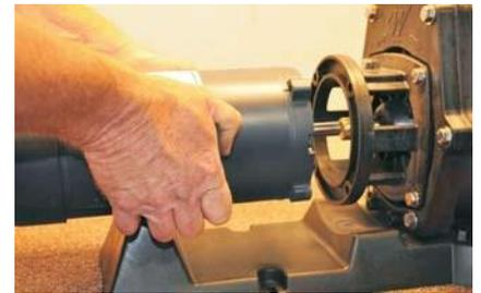
9. Slide the motor toward the pump until it touches the motor adapter.
