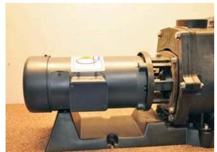
10. Install the four 3/8-16 motor bolts through the motor adapter into the motor and tighten.
