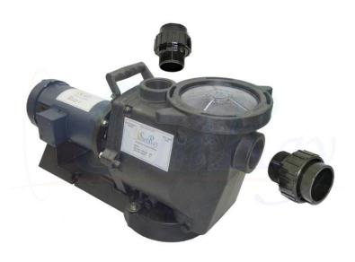
SunRay manufactures a variety of DC powered centrifugal surface pumps. Among the most popular are the SolFlo series pool pumps. They will replace almost any AC powered pool pump and because they get their power from the sun, you will save on your power bill. They are available from 1/2 to 3 horse power and operate on 100 to 3000 watts of DC power.
