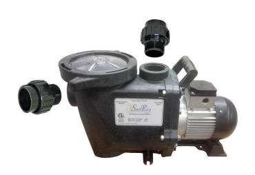
The SloFlo2+ series pump are single stage centrifugals constructed from high performance thermoplastic. They are extremely resistant to mineral and algae deposits while providing outstanding strength and durability. For added protection there is a basket strainer incorporated into the suction side of the pump. Simplicity is a key feature of the SloFlo2+ series pumps. They are simple to install and field servicing is easily accomplished without the use of specialized tools.
